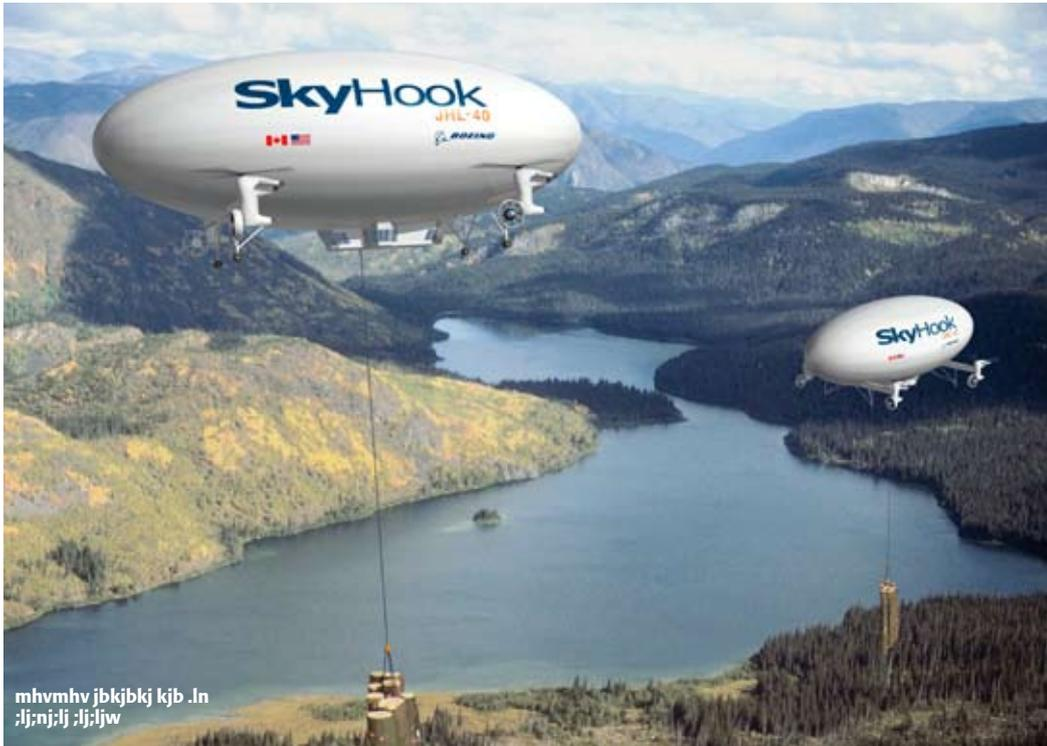
◀ The JHL-40, which will be developed and built by Boeing, combines a neutrally-buoyant semi-rigid helium envelope with four Chinook helicopter rotors. The inert gas provides enough lift to support the aircraft, leaving the rotors to lift cargo – 40t at a time – and propel it at up to 70 knots (130km/h) over its range of 320km.
